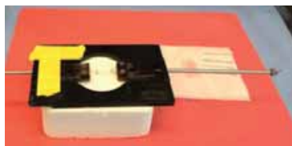
The first cracks were observed when the applied strain reached about 5%.
