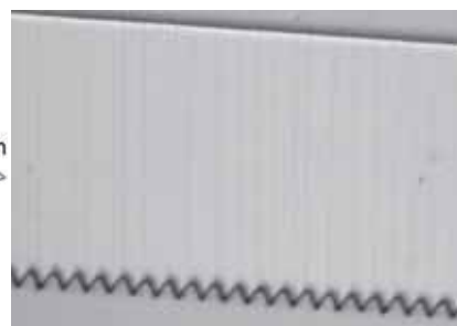
Fig.3 Nanochannels (tunnel cracks) connecting the two microchannel reservoirs were created within the bonded oxidized layer in response to a tensile strain.
